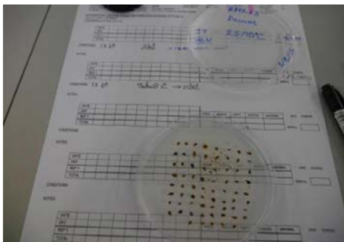
Germination test sheet and the Daucus spp. seed set up on an agar plate for testing.
