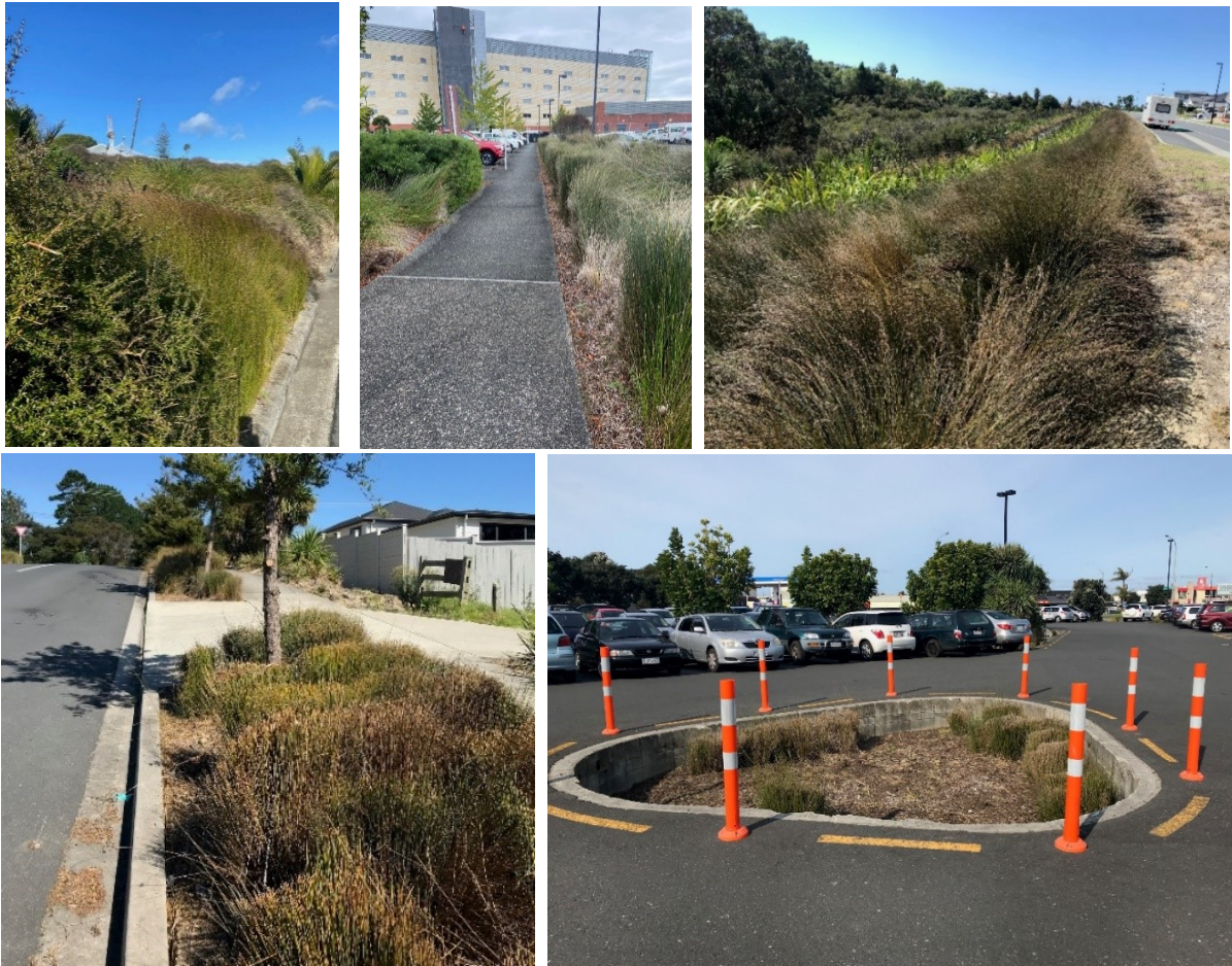
Figure 7. Opportunities and challenges when growing oioi in urban stormwater and garden environments. Top left & middle: Oioi has been cut almost vertically and mainly along the edge, so that leaves do not flop onto the pavement but very little bare ground is exposed (reducing weed invasion) and survival is not impaired. The plants are sometimes topped high create a ‘hedged’ aesthetic and keep sight lines open 126 . Top, right: The landscaped edge to riparian planting at Orewa (North Auckland) does not need trimming; the side abutting the grass verge is maintained by mowing of grass and some spraying along the edge. Bottom, left: Severe cutting of this berm risks killing the oioi. Bottom, right: Heavily trimmed oioi in this Panmure (Auckland) raingarden eventually died.
