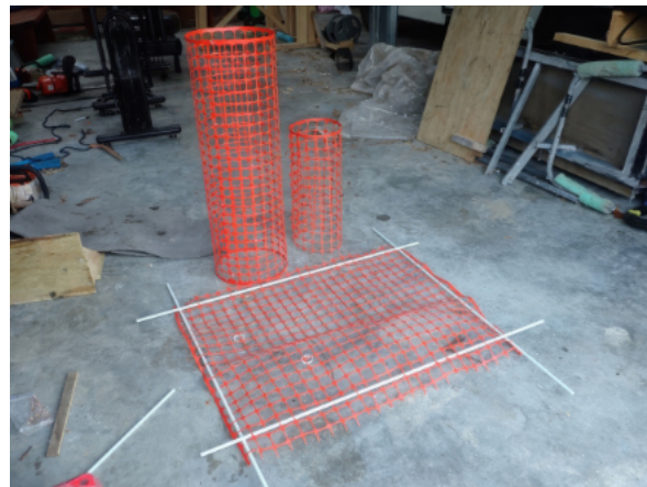
Figure 4. Showing the uses of the mesh, either flat or rolled into a guard.
